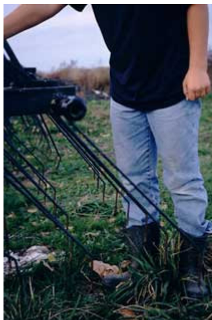
Peter Martens showing the possible angle adjustments on a Kovar coil tine harrow with 45 degree teeth.
