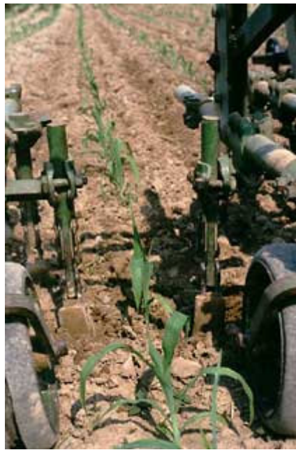
Front view of John Deere front cultivator with trip shanks and a homemade track digger with Danish tines.
