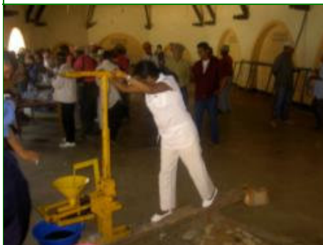
The national coordinator of the PLAE testing the ram press to extract Jatropha oil
