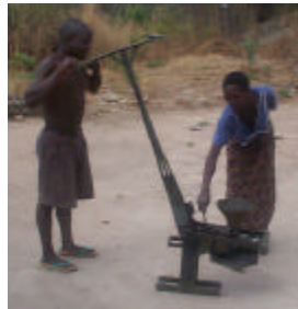
The Bielenberg ram press for manual oil extraction
