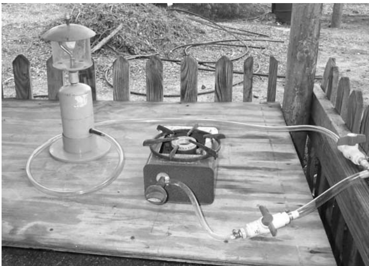
Figure 5. Gas from the storage container can be used in salvaged gas stove burners or any similar locally fabricated device. Gas may also be used in any common pressure lamp after its fuel orifice has been modified.
