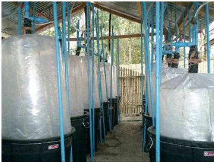
Photo 2: The inverted containers for collecting the biogas by water displacement
