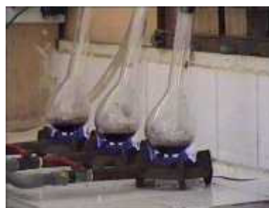
Photo 96. Using the biogas to digest samples for Nitrogen analysis
