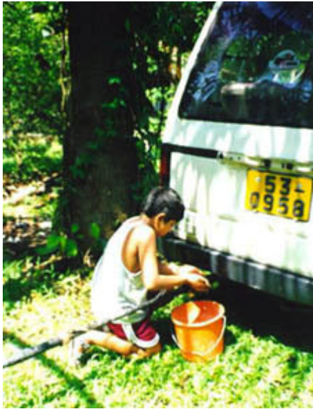
Figure 9. Connecting a hose to the exhaust pipe of a car, in order to fill the plastic bag with exhaust.
