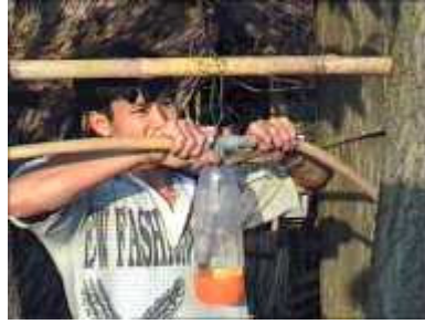
Photo 50. Joining the other end of the PVC "T" to the plastic hose that goes to the reservoir bag
