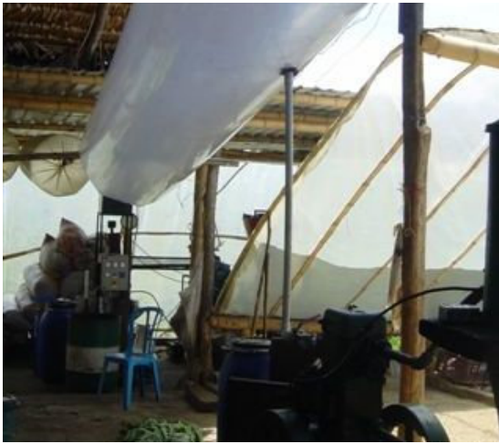
Photo G7: A similar system is used to store the gas in the reservoir of 7m 3 that will fuel the Lister engine running in " dual-fuel" mode.
