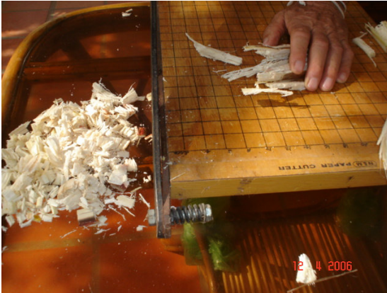
Photo G5: Sugar cane bagasse after chopping with a guillotine. A way has to be found to mechanize this process and still achieve the necessary reduction in size
