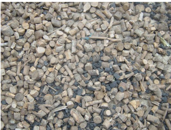
Photo G3: The chips from the waste wood and bamboo that will be the feedstock for the gasifier
