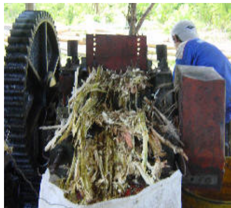
Photo G4: The 3-roll crusher used to extract the juice from sugar cane. This residue can be chopped into smaller pieces (Photo G5) but because of the lower density is not a suitable fuel for the "Ankur" gasifier which has been designed specifically to use wood chips.
