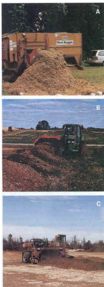
Fig 4. Techniques for large-scale composting include (A) mixing poultry litter and agriculture by-products in a feed mixer for passive aeration composting, (B) using a tractor-pulled windrow turner to mix cannery wastes with sawdust and municipal leaves, and (C) turning poultry litter using a self-propelled windrow turner.
