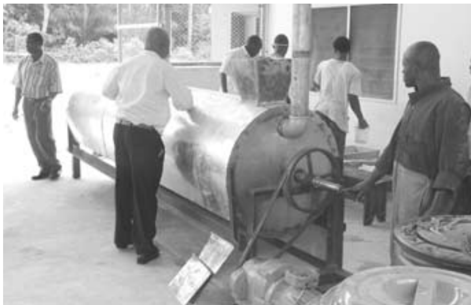
Prototype of rotary dryer at IITA Onne.
