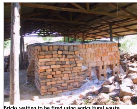
Bricks waiting to be fired using agricultural waste
