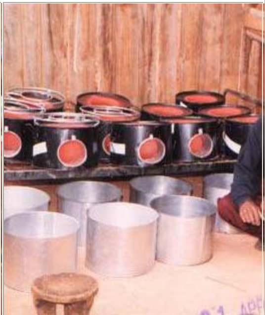
Richard Njagu with New Stove Design April 2003 12.5" dia x 9" h, 6" exit, 9" dia firebox, 5" dia fuel feed Cement and pumice construction with pumice insulation
