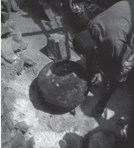
Figure 4 Each stove is custom made. Measurements of the vessel are taken based on the diameter of the cooking vessel. (photo: Peeyush Sekhsaria)
