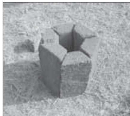
Figure 3 Pumice/clay combustion chamber
