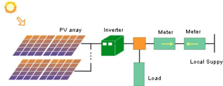
Fig.1. Single inverter Grid Connected System.
