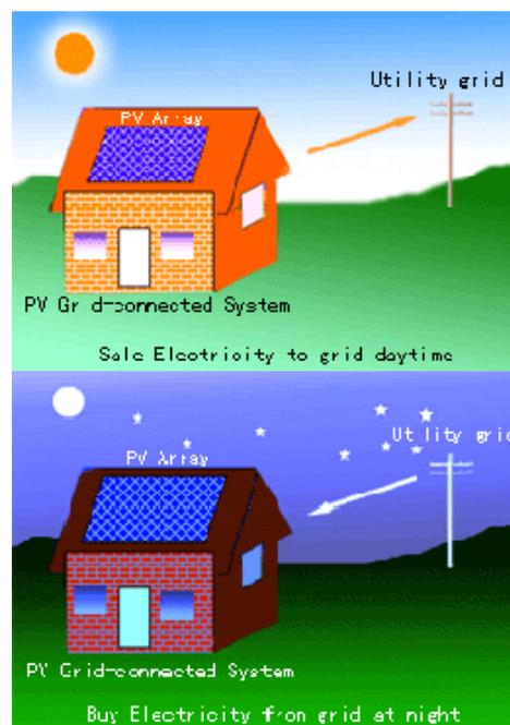
Grid connected system avoid the need for electricity storage in batteries by essentially using the utility as a battery system. When your solar or wind system produces more electricity than you need, the excess is sold back to the utility. When your system doesn't
